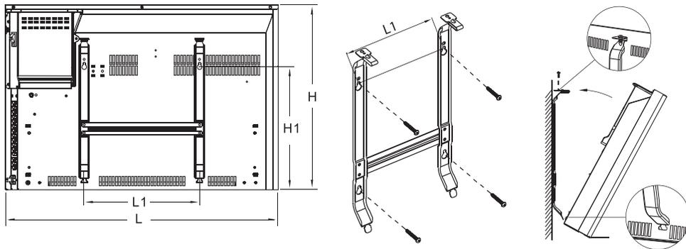
1. Insert the bracket (into the hole), turn it 90° anti-clockwise to fasten the screw.
