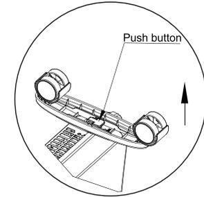
Push the button up to remove the caster
