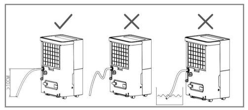
Attention: The external water pipe must not be too long (the recommended length is less than 0.6 meters). The height of the end of the water pipe must be more than 10cm lower than the height of the water outlet. The water pipe must be kept smooth, otherwise the water may not be drained normally.
