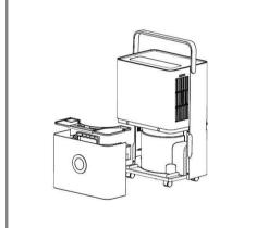
Close the tank cover, and rotate the water tank handle down, then put the water tank gently and put it back in the right place to restart dehumidifier.
