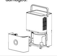
Clean the filter and the frame at lease once per two weeks simply with cold or warm water, do not use chemical solvents or hot water.
